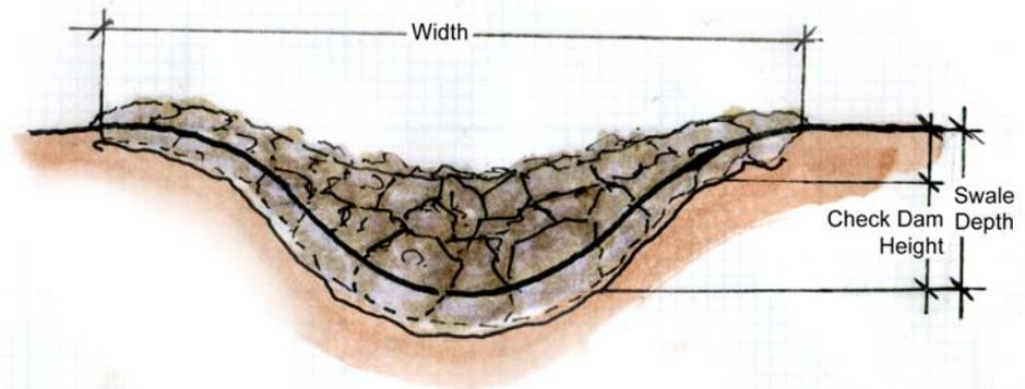
on their, size, shape and weight. The upstream face should be more gradual (approximately 66% or 1.5-2:1) than the downstream face.
