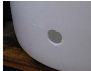
4. Remove any plastic shavings that may have fallen into the barrel.
