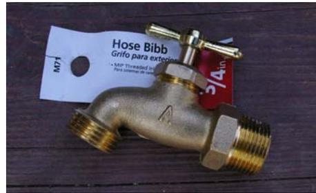
2. Point the spout downwards and seal the joint with silicone caulking.
