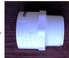
3. Tightly wrap the threaded end of the adapter with pipe tape and screw overflow spout into 1 7/8" hole at the top left-hand side of the barrel. Point the spout downwards (and away from your foundation) and seal the joint with silicone caulking.
