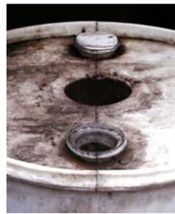
3. Next, drill a 1 7/8" hole in the left side of the barrel one inch from the top. Then, drill a 1 1/8" hole at the base of the front of the barrel for the spigot.
