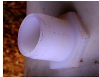
2. Firmly push the flexible tubing onto the adapter to attach. Slide the adjustable clamp or zip-tie into place and tighten.
