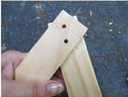
Figure 2: Holes through overlapped ends same time (Figure 2). It isn't important exactly where the two holes are so long as they go through both boards and are far enough from the edges not to break through.
