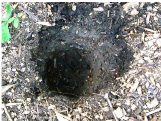
Figure 5: Completed perc test, 30 minutes after start
