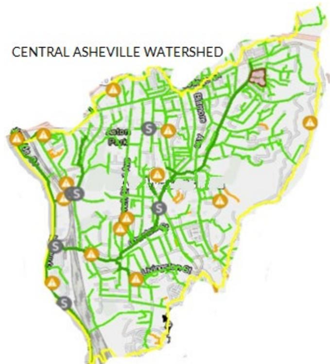
Figure 13 MSD Sanitary lines in the CAW and reports of SSO (denoted by an S) and Odor problems (denoted with triangles) in the past three years.
