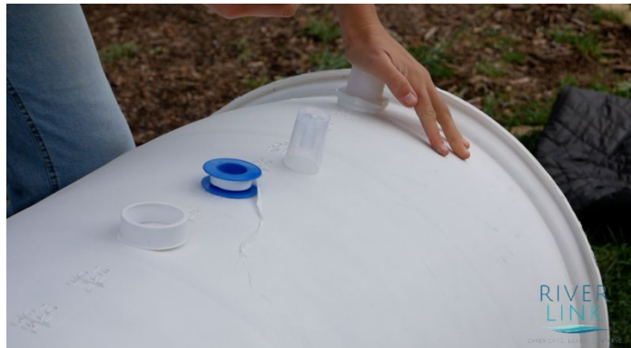
Figure 22 Inserting threaded nylon adapter
